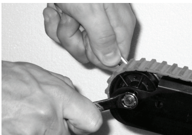
Figure 7 – Use wrenches to apply tension to the belt
