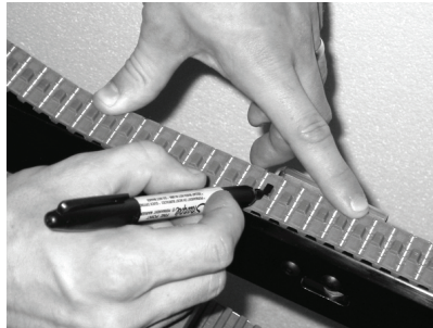
Figure 4 – Mark a belt tooth for reference
