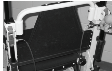
Figure 12 – Attach one side of the new cable
