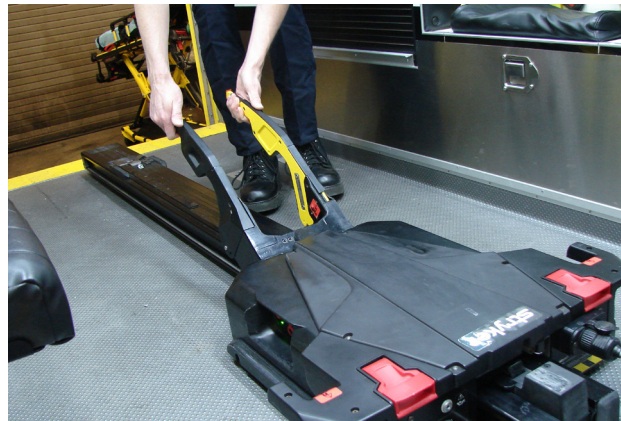
Figure 34: Pull Trolley Out
