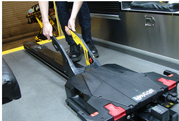
Figure 34: Pull Trolley Out
