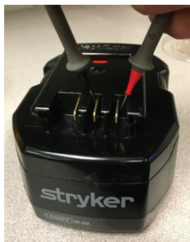
Figure 2 – Check the battery voltages (cot battery shown)
