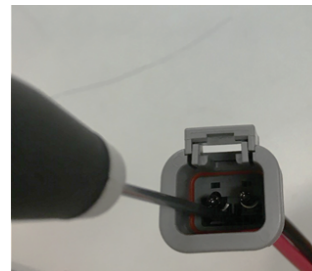
Figure 5 – Depress the connector latches
