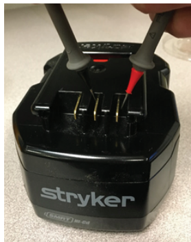
Figure 2 – Check the battery voltages (cot battery shown)
