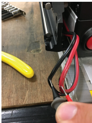
Figure 8 – Check the copper wire voltage
