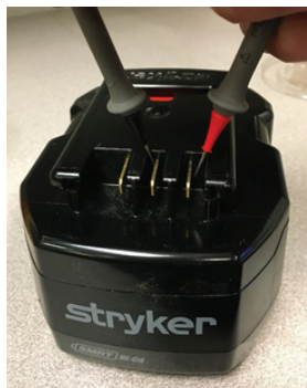
Figure 2 – Check the battery voltages (cot battery shown)
