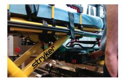
Figure 31 - Raise the lifting arms to the highest position
