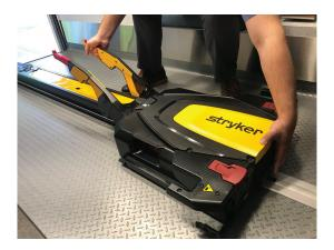
Figure 27 - Press trolley release button
