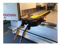
Figure 48 – Guide the trolley out of the vehicle
