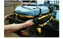
Figure 40 – Press and hold the release lever
