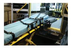
Figure 30 - Lock wheel pins into position
