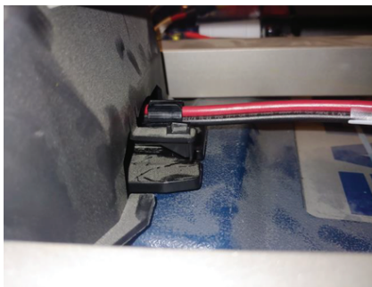
Figure 8 – Push the connector into the cavity
