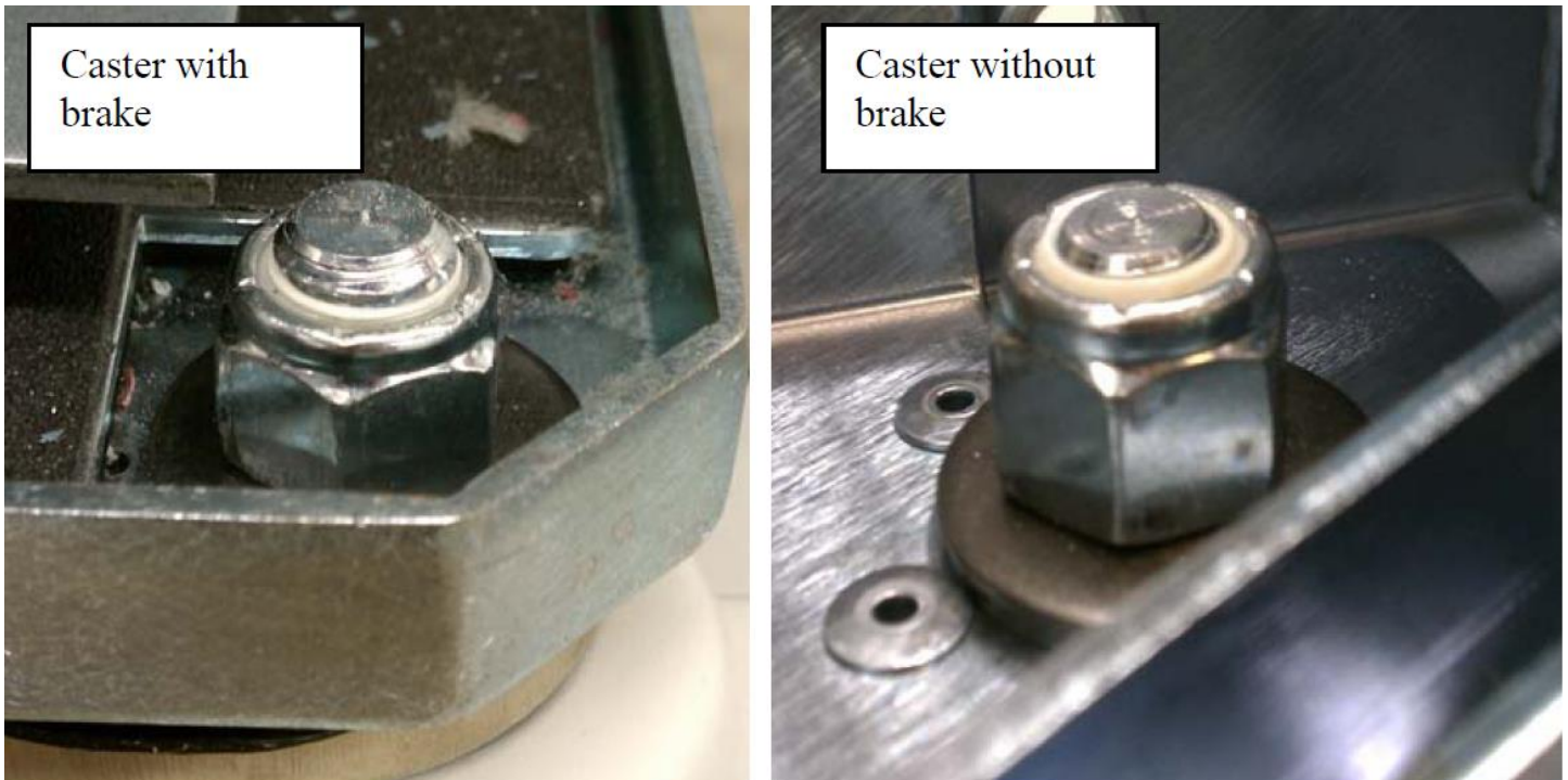
Figure 4. Position of nut on caster stem
