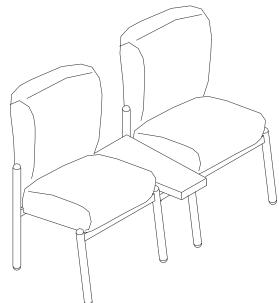
4. With the Ganging Brackets attached to each chair, place the Filler Table Top on top of each bracket, as shown.
