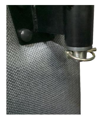
9. Thread (1) Knob 207007 into the table mount and tighten until snug.
