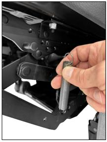
5. Unhook the bottom of the spring from the recline mechanism as shown. Discard the spring.
