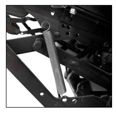
4. Carefully grasp the upper part of the spring to remove the spring hook form the recline mechanism as shown.
