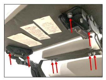
11. **300 Series only**: Using a Ratchet and 7/16" Socket, remove the two nuts on the front edge of the seat frame that secure the seat cushion to the recline mechanism.
