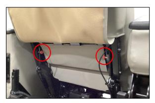
26. Snap the plastic sleeve grommet of the cable into the top of the release head.
