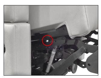
34. Reinstall the centerboard and the legrest using (8) Lock Washers and (8) Nuts. Tighten all hardware using applicable tools.
