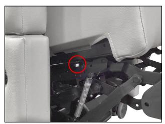
12. From the foot side use a Ratchet, 7/16" Socket, and 4mm Hex Wrench, remove the bolts, washers, and nuts from the right and left side securing the recline mechanism to the base frame. Repeat for the head side. Save the bolts, washers, and nuts.
