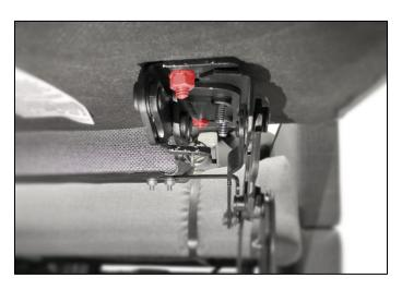
4. Using a Ratchet with 7/16" Socket, remove the faulty footrest safety device from the recline mechanism. Discard the safety mechanism and the bolts (left side shown in images).
