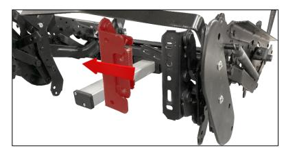
5. Using a Ratchet with 7/16" Socket, install the new footrest safety device onto the recline mechanism using the supplied bolts. Tap the safety device down using a Rubber Mallet before tightening completely. Repeat for opposite side.
