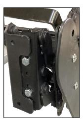
6. Using a Ratchet with 7/16" Socket, secure the footrest to the recline mechanism, reusing the washers and nuts.
