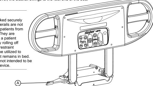
To disengage the rail, push in the blue release handle (A) and swing rail down to desired height. Tuck away siderails by pushing the rails under the bed. Rails must be in the full down position before they can be tucked.
