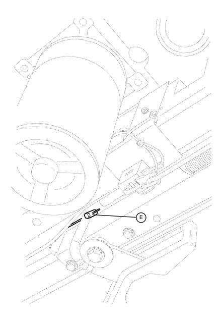
6. Using two 3/16" hex socket drivers, loosen the bolt in the cable retainer (E) and slide the retainer off the cable. Pull the cable out of the bed.
