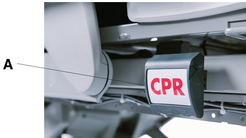
Figure 16 – Activating the CPR release handle
