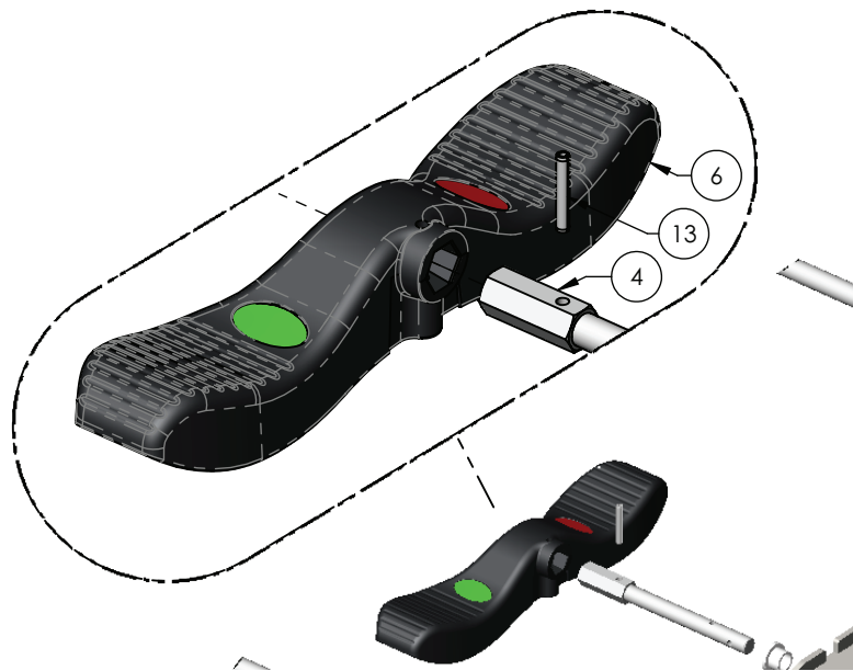
Figure 2 – Brake pedal replacement
