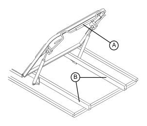
Squeeze handle (A) for pneumatic assist in lifting the Fowler to the desired height. Remove hand(s) from handle when desired height is achieved.
