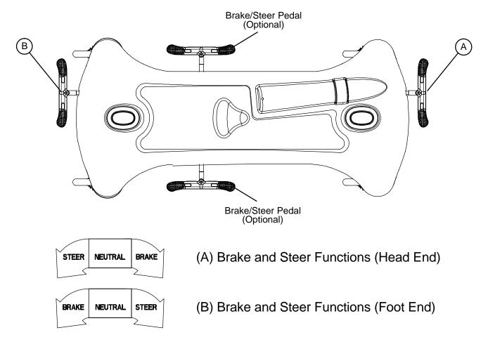
To engage the brakes from the head end of the stretcher, push fully down on the left side of pedal (A). To engage the brakes from the foot end of the stretcher, push fully down on the right side of pedal (B).
