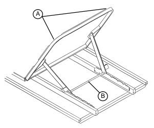
Lift up on the Fowler handles (A). The brace assembly (B) will fall into position as the Fowler is raised to the desired height.
