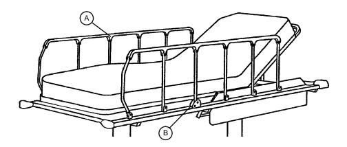
To engage siderails: Pull up siderail (A) and raise to full up position so that latch (B) engages.
