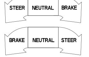
Pedal (D) - Brake and Steer functions (head end)
