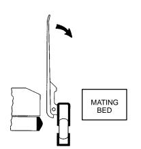
3. When the transfer board is fully raised, it can be pivoted downward onto the surface of the mating bed or stretcher.
