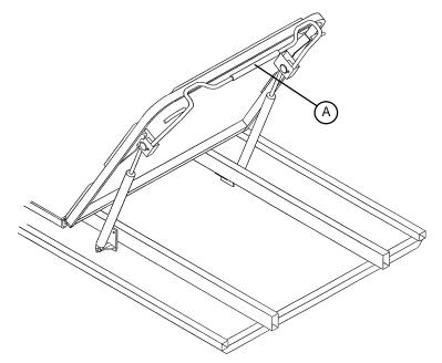
Squeeze handle (A) for pneumatic assistance in lifting the Fowler to the desired height. Remove hand(s) from handle when the desired height is achieved.
