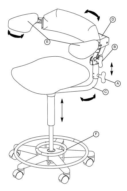
To raise or lower the height of the back rest assembly, turn knob (A) counterclockwise, raise or lower the back rest and turn the knob clockwise to tighten it and secure the back rest.
