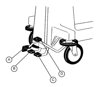
A Press fully down to engage four wheel brakes. Lift fully up to release brakes.
