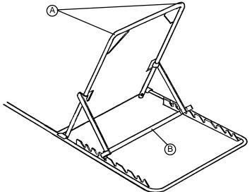
Lift up on handles (A). The brace assembly (B) will fall into position as the Fowler is raised to desired height.
