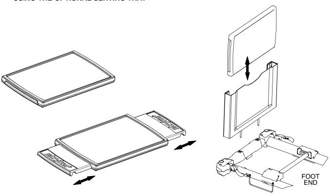
Pull out on either end of the serving tray to extend it to the proper width to fit on top of the stretcher siderails. To store the serving tray in the optional serving tray holder/foot board, push in both ends of the serving tray and slide it into the holder.
