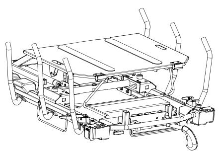
To prop the foot end of the Knee Gatch up, lift up the end of the Knee Gatch, allowing the prop rod to swing down and engage in the bracket. To release the prop, lift up on the end of the Gatch, swing the prop rod toward the head end of the bed to disengage the bracket and lower the foot end.
