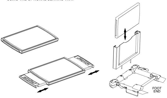
Pull out on either end of the serving tray to extend it to the proper width to fit on top of the stretcher siderails. To store the serving tray in the optional serving tray holder/foot board, push in both ends of the serving tray and slide it into the holder.
