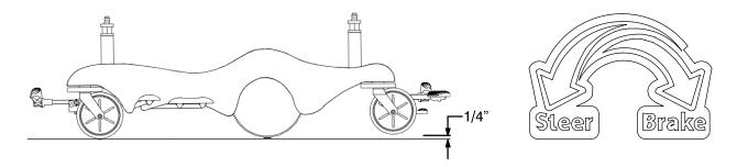
When the brake/steer pedal is in the **steer** position, the foot end casters are elevated approximately 1/4" and the stretcher rests on the two head end casters and the two Big Wheels. This provides increased mobility and ease of steering the stretcher.
