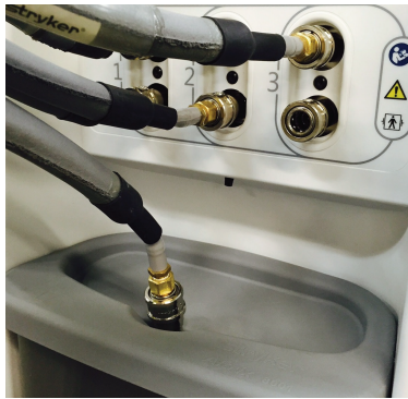
Figure 1-30: Bottom hose end in the lid of the reservoir
